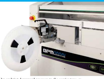
by applying downward pressure to the carrier tape, resulting in precise presentation of small components to the APS nozzle. Controlled tension between the input reel and feeder provides fluid carrier tape movement, producing uninterrupted production programming.
